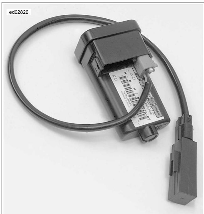
Figure 3-15. HFISM and Antenna
