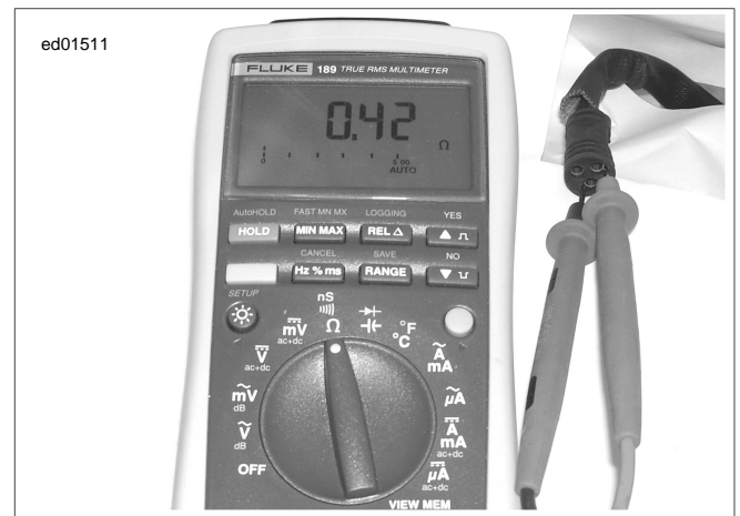
Figure 1-19. Check for Stator Resistance (Typical)
