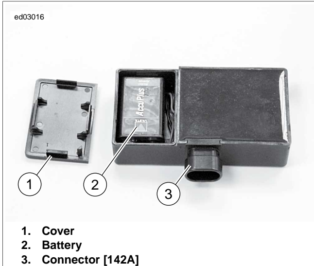
Figure 3-37. Battery Compartment (Early Style Siren)
