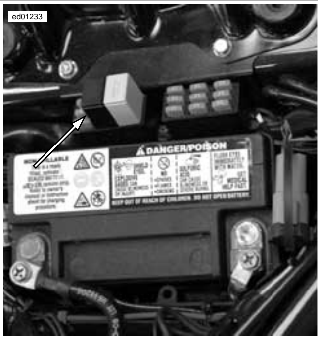
Figure 4-27. System Relay (FXCWC)
