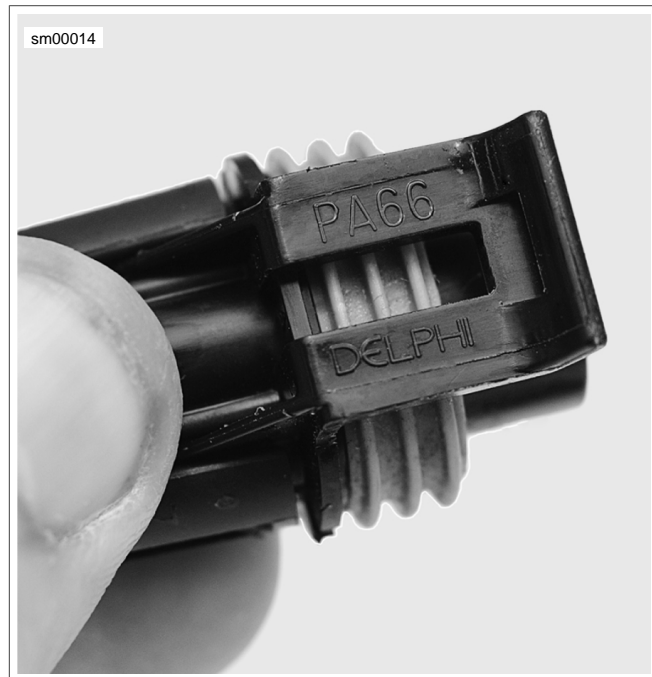
Figure A-10. Delphi Connector: Socket Housing Latch
