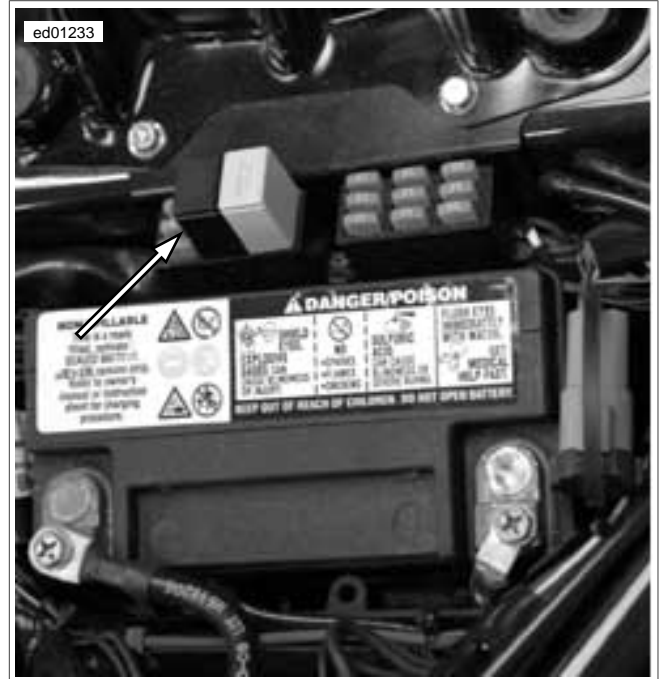
Figure 4-30. System Relay (FXCWC)
