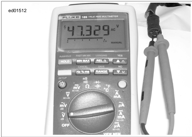
Figure 1-20. Check Stator AC Voltage Output (Typical)
