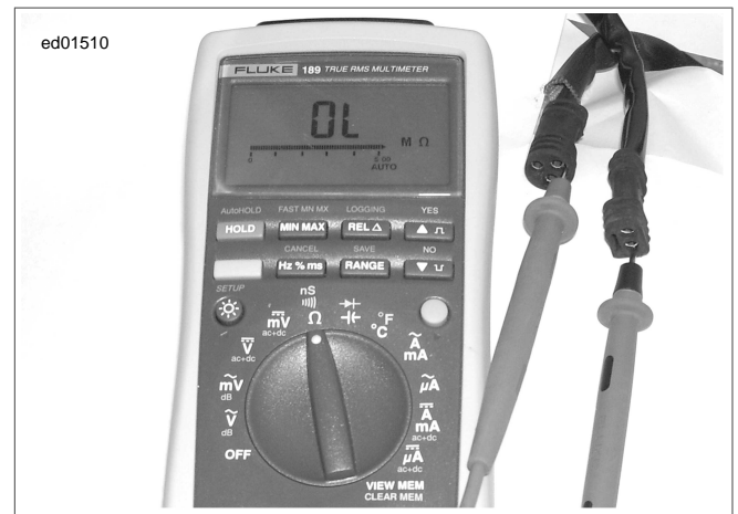
Figure 1-18. Test for Grounded Stator (Typical)
